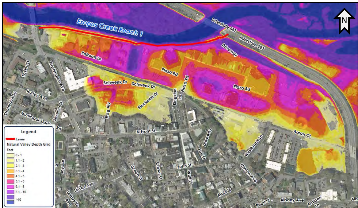
Figure 4: Natural Valley Procedure Flood Depth Grid
